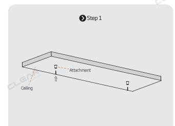
Mount the attachment of cable couplers to the ceiling with sufficient load-carrying capacity and tighten them with screws.
