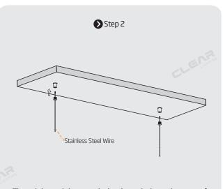
Thread the stainless steel wire through the male screw of cable couplers and then connect to the mounted attachment of cable couplers.
