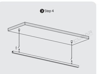
Thread the stainless steel wire through the bushing of cable gripper.
