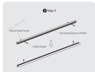
Insert the screw into the serrated aluminum profile to lock with the cable gripper sliding from the bottom slot of serrated aluminum profile.
