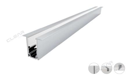
Specialized for the LED Flex Linear light, it was developed by combining the advantages of 6063 aluminum and elastic serrated tape. The inside elastic serrated tape as the grabbing force to keep continuous strong clamping force on the light body and protect the light from the damage caused by the large friction in the process of installation and dismantlement,
