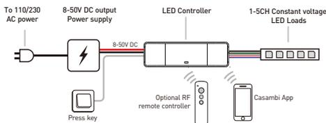
This model supports 1-5 channel application from single color to RGB+CCT, please refer to following diagram for multiple application output wiring.
